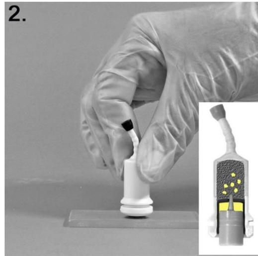
For activation of the ORBIS Cap press the plunger on a hard and plane surface to the end into the ORBIS Cap.
